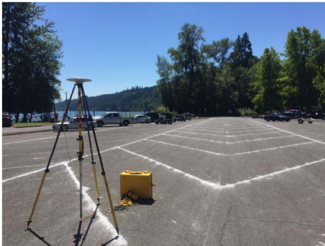
Figure 3. PK nail in the middle of Willamette Park Boat Launch parking marks survey monument PH3. It was land-surveyed by DEA and marked with pink survey tape. Photo shows survey equipment set-up over PH3.
