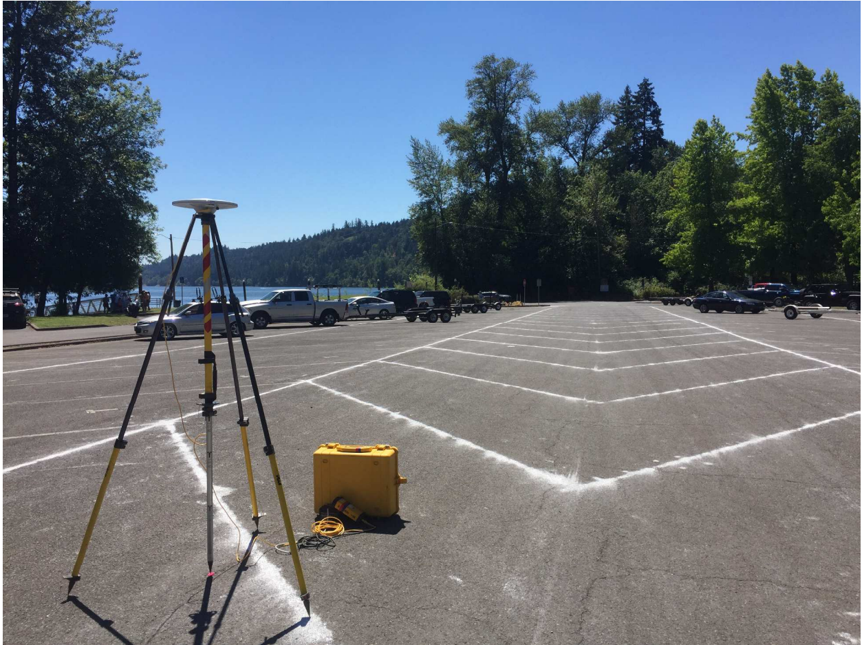
GNSS Setup on PH3
